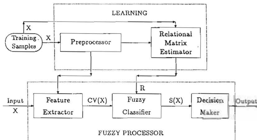
Fig. 1. Block diagram of the multivalued recognition system [11].
