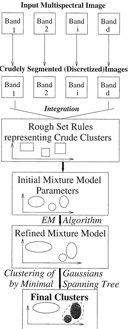
Fig. 1. Block diagram of the proposed clustering algorithm.
