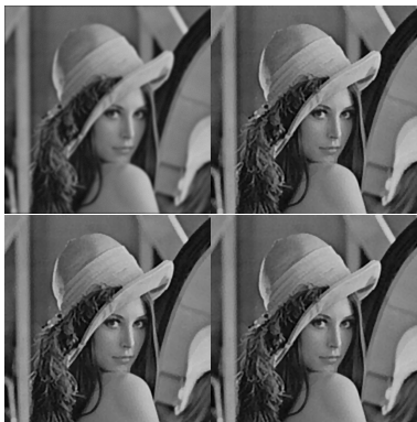
Figure: Illustrates results of deblurring technique with various regularization methods. Top row: noisy and blurred input image and TV regularization (PSNR = 29.93dB, SSIM = 0.9224). Bottom row: using BTV (PSNR = 29.95dB, SSIM = 0.9224) and Morphologic regularization (PSNR = 30.05dB, SSIM = 0.9248).
