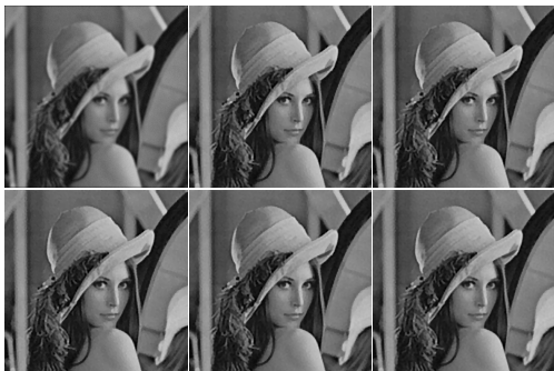
Figure: Illustrates results of SR technique with various regularization methods. Top row: SR image using Bicubic interpolation, TV (PSNR = 29.43dB, SSIM = 0.9077) and BTV (PSNR = 29.47dB, SSIM = 0.9080) regularization. Bottom row: using geodesic (PSNR = 29.48dB, SSIM = 0.9082), Morphologic (PSNR = 29.55dB, SSIM = 0.9106), and Adaptive morphologic method (PSNR = 29.59dB, SSIM = 0.9107).
