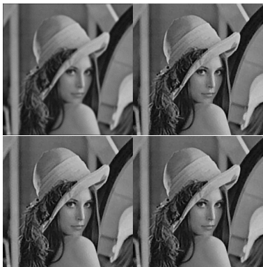
Figure: Illustrates results of SR technique with various regularization methods. Top row: SR image using Bicubic interpolation and TV regularization (PSNR = 29.43dB, SSIM = 0.9077). Bottom row: using BTV (PSNR = 29.47dB, SSIM = 0.9080) and proposed Morphologic regularization (PSNR = 29.55dB, SSIM = 0.9106).
