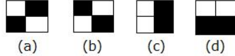
Figure 3. Four structuring element (a)-(d) with center as the first element used to find the images containing the portion of skeleton in the respective direction.
