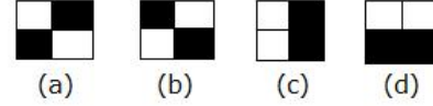
Figure 3. Four structuring element (a)-(d) with center as the first element used to find the images containing the portion of skeleton in the respective direction.
