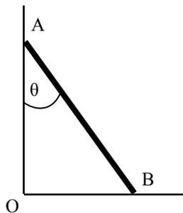
Assume the coefficient of static friction  $\mu_s$  is the same at both the surfaces of contact. Determine the smallest value of  $\mu_s$  for which the equilibrium will be maintained.
