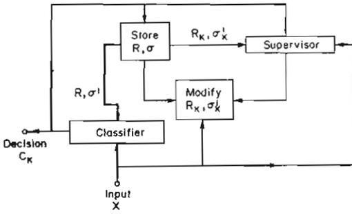
Fig. 1. Block diagram of an adaptive vowel recognition scheme.
