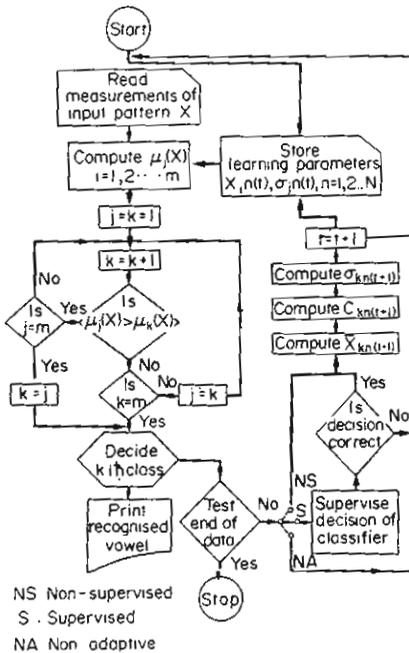
Fig. 5. A flow chart for the recognition system.
