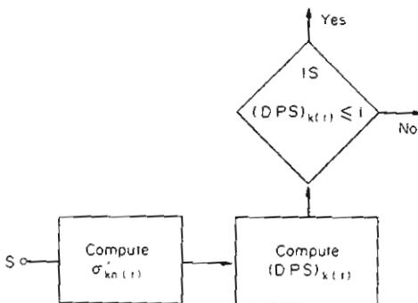
Fig. 6. Block diagram of supervisor for self-supervised learning algorithm.
