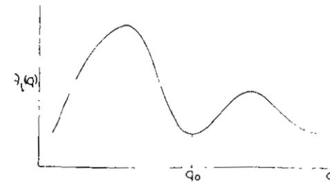
Fig. 1. Graph showing index of fuzziness values vs. crossover points  $q_0$  is optimal.
