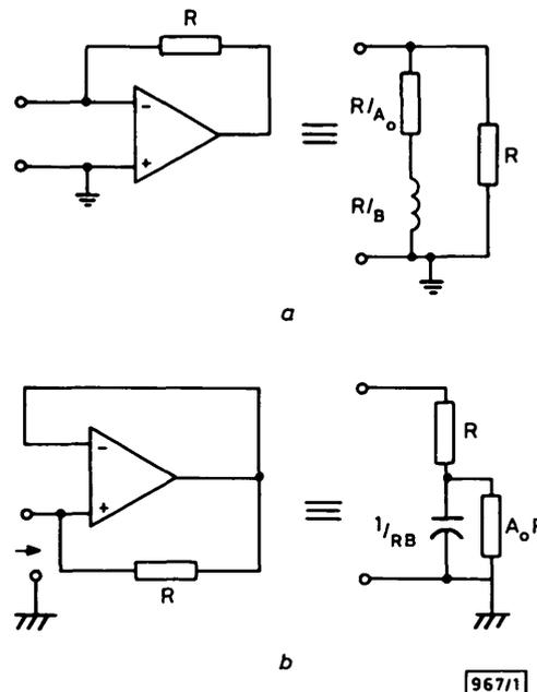
Fig. 1 Lossy simulated inductor (a) and lossy simulated capacitor (b) using the amplifier pole
