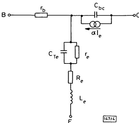
Fig. 4 Equivalent circuit of transistor
