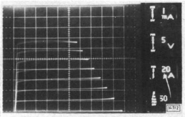
Fig. 2 Static  $I/V$  characteristics of GaAlAs/GaAs heterojunction microwave bipolar transistor
