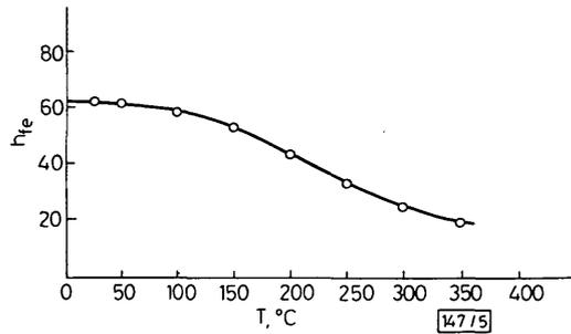
Fig. 5  $h_{fe}/\text{temperature}$  characteristic for heterojunction transistor
