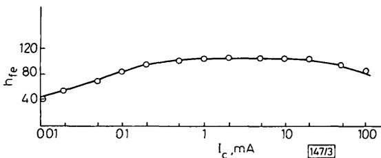
Fig. 3  $h_{fe}/I_C$  behaviour of transistor
