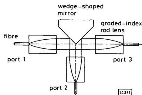
Fig. 1 Schematic diagram of tee coupler
